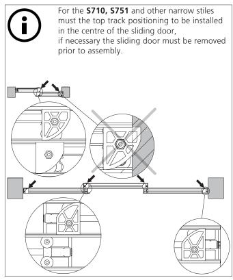
**5**\_ Positioning examples for the top track positioning
