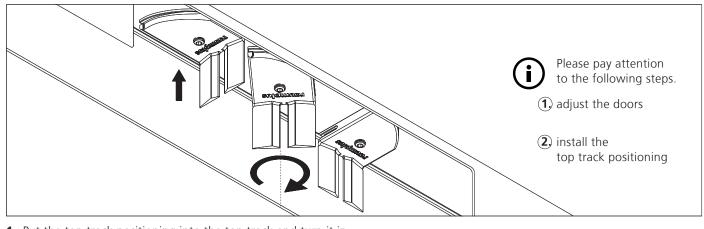
**1\_** Put the top track positioning into the top track and turn it in
